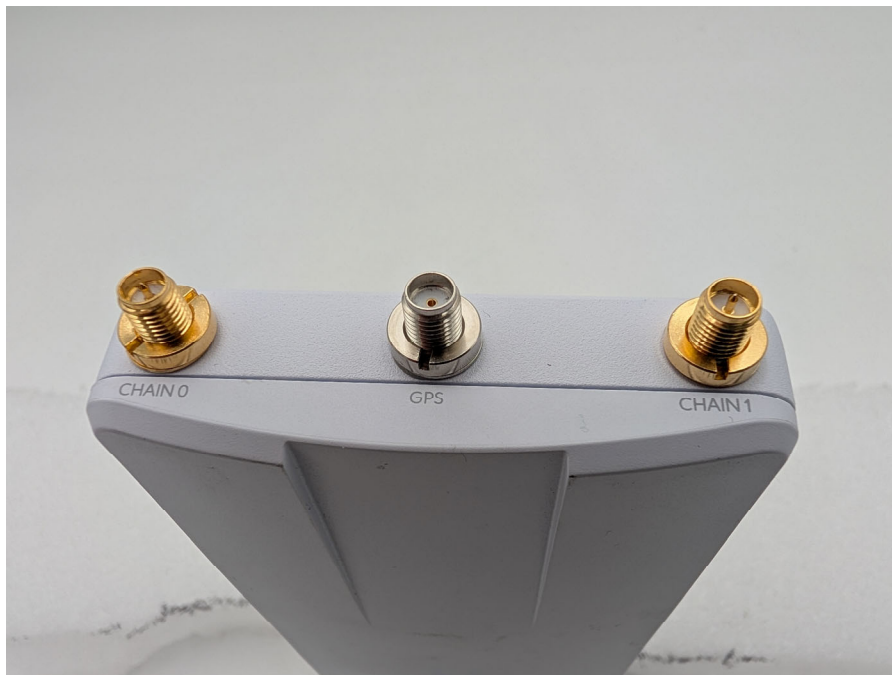
Photograph 6: Close Up Top View of Antenna Ports
