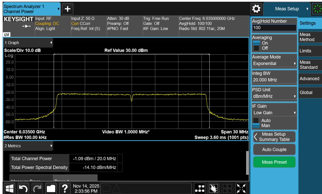
Plot 11: Power and PSD for Standard Power – 6035 MHz
