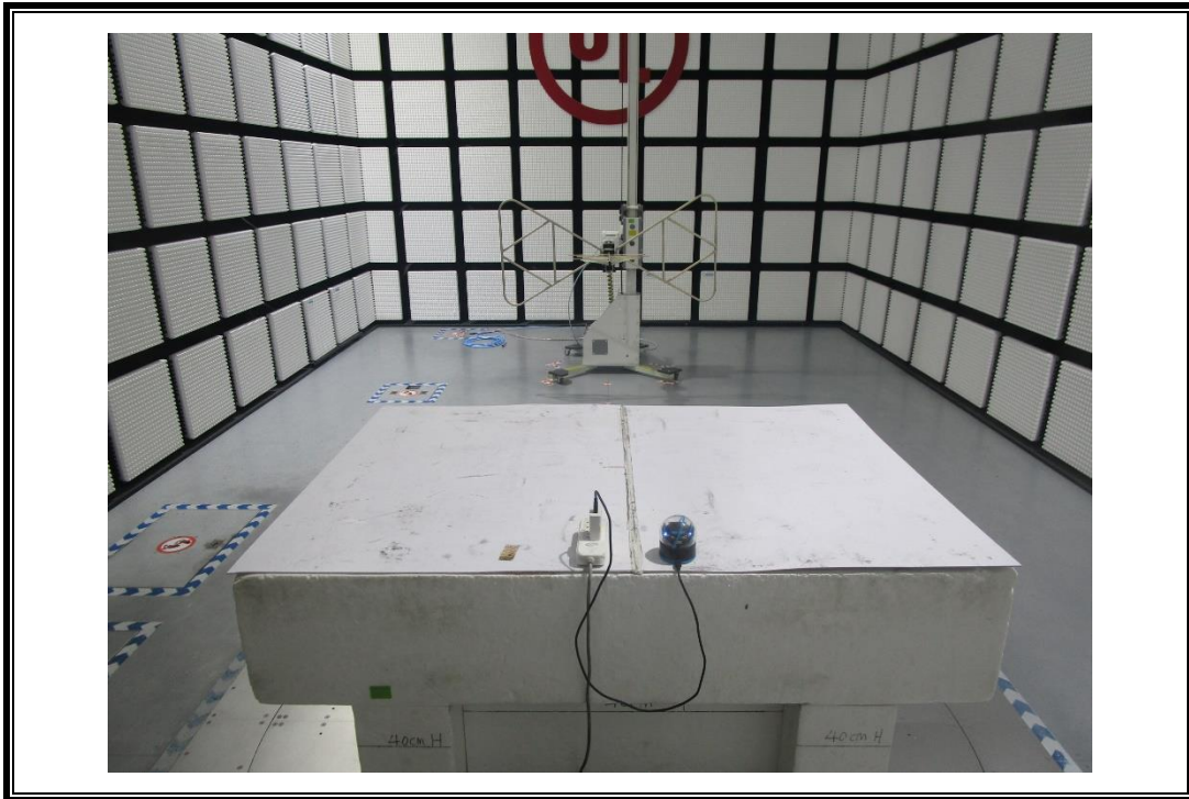
RADIATED EMISSIONS MEASUREMENT SETUP (30MHz ~ 1 GHz)
