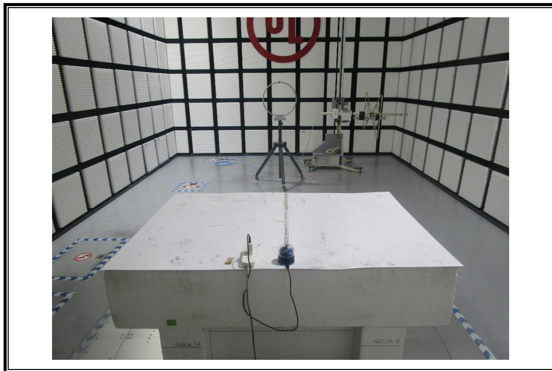
RADIATED EMISSIONS MEASUREMENT SETUP (Below 30MHz)
