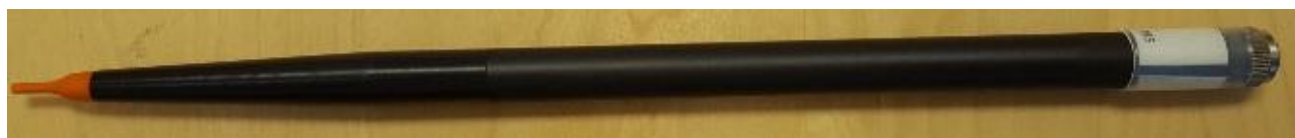
Figure 1 – MVG COMOSAR Dosimetric E field Dipole
