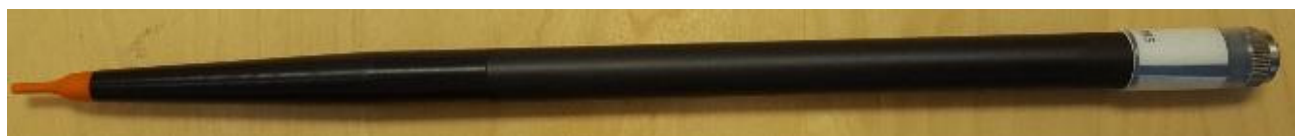
Figure 1 – MVG COMOSAR Dosimetric E field Dipole
