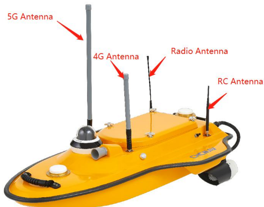
Figure 2-4 Install the accessories on the boat
