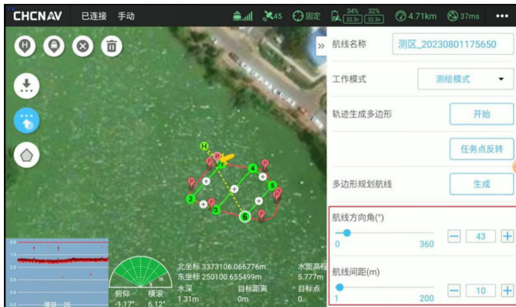
Figure 11.21: Adjusting the course direction angle/course spacing
