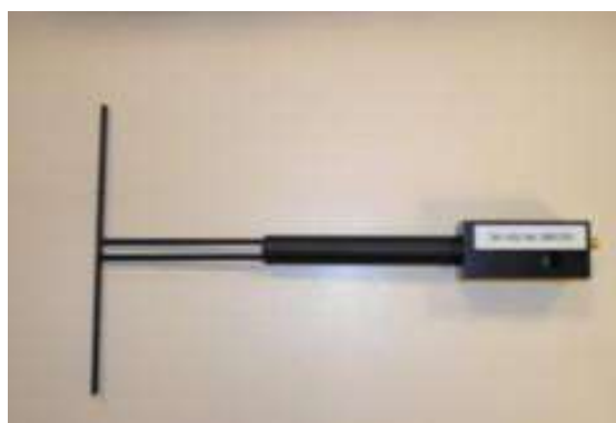
Figure 1 – MVG COMOSAR Validation Dipole
