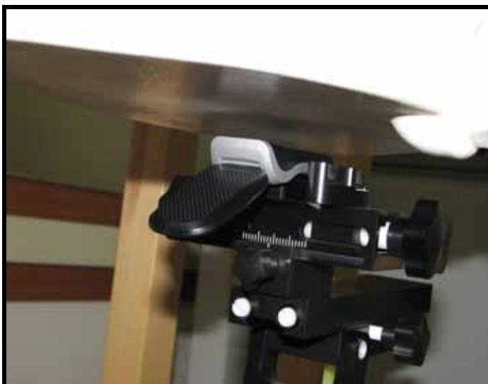
Figure 9.5 Muscle SAR Test Setup -- 15mm Distance Position --
