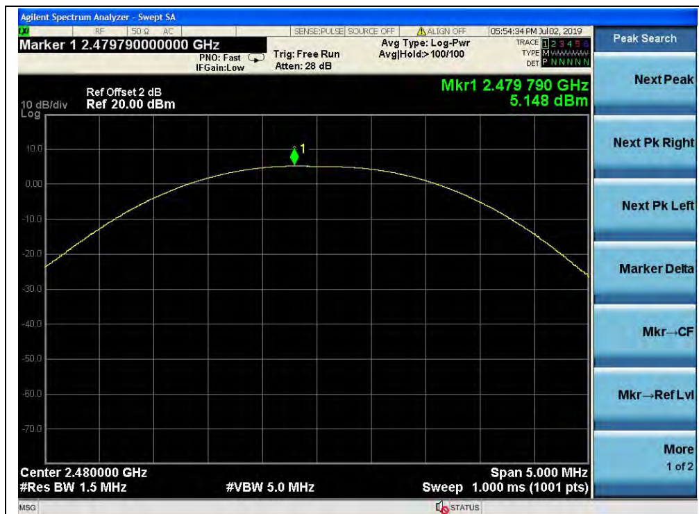
(GFSK, Channel 78, 2480MHz)
