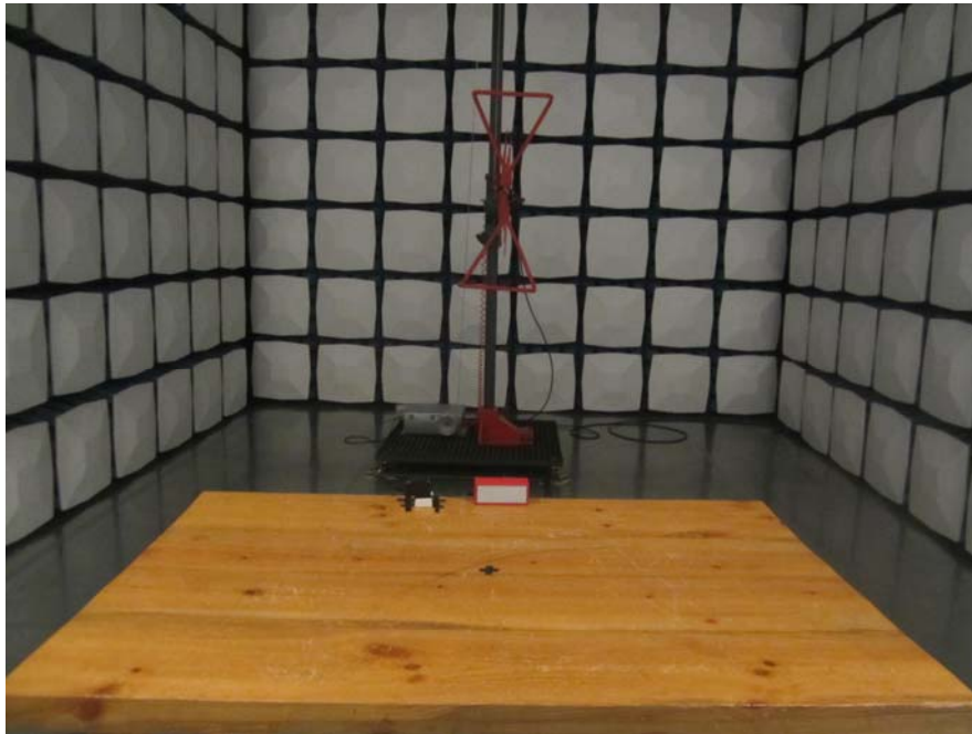
Radiated Emission -Front View (Below 1GHz)
