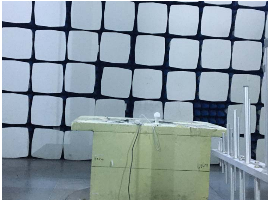
Radiation Emission Test Setup (30MHz to 1GHz)
