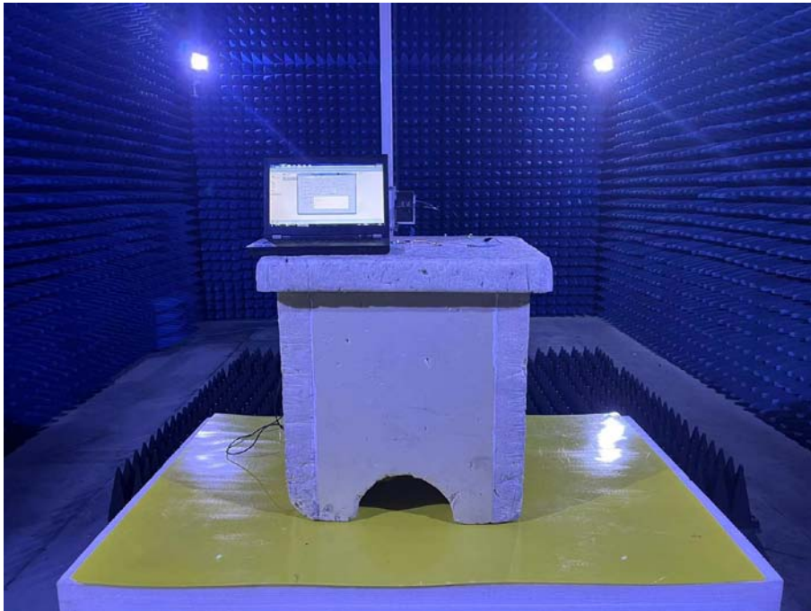
Photo of Radiated Emission Measurement Above 1GHz
