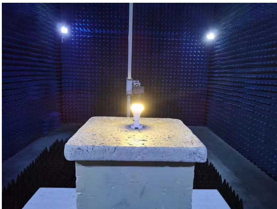
Photo of Radiated Emission Measurement Above 1GHz
