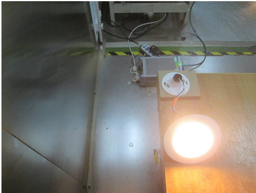
Conducted Emissions - Side View
