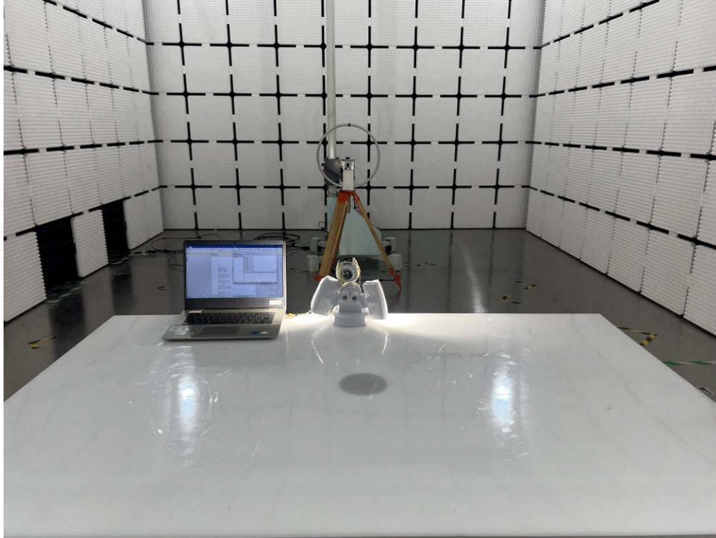
Radiated emission (30-1000MHz)
