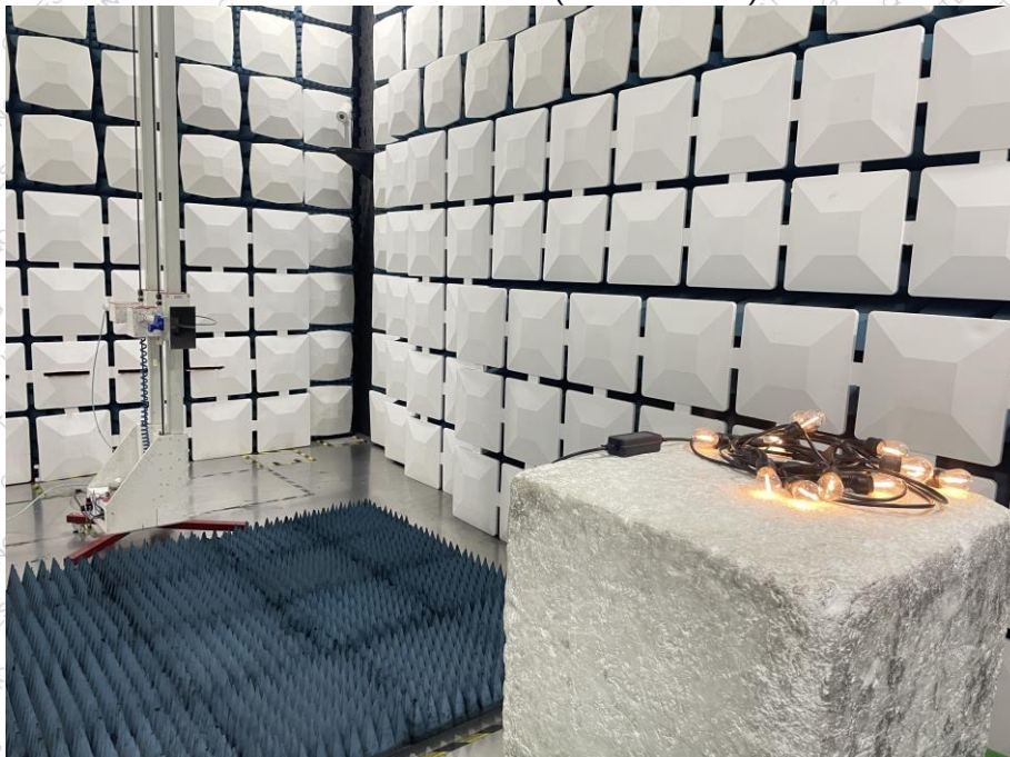
Radiated Emissions (Above 1 GHz)
