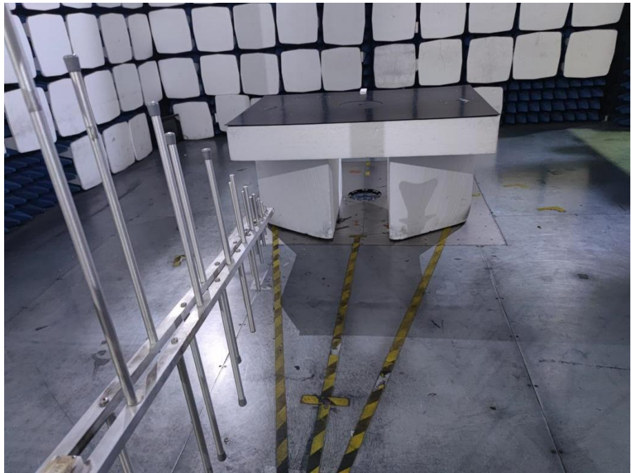
Radiation Emission Test Setup (30MHz to 1GHz)
