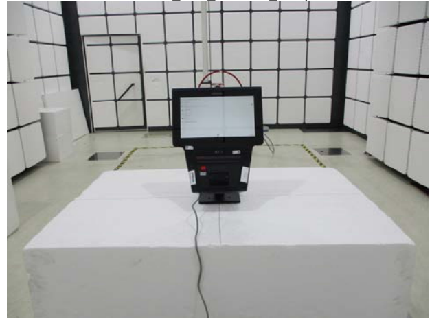
P15.225 NFC Radiated variant Setup
