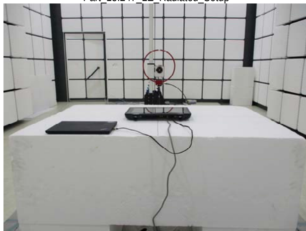
Part 15.247 LE Radiated Setup
