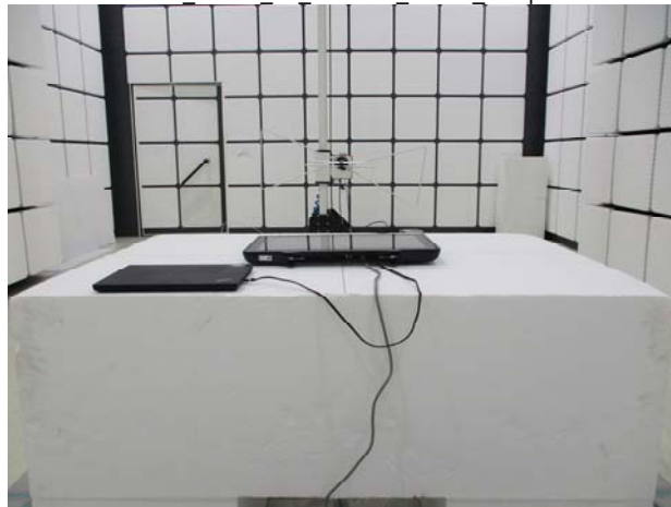
Part 15.247 LE Radiated Setup
