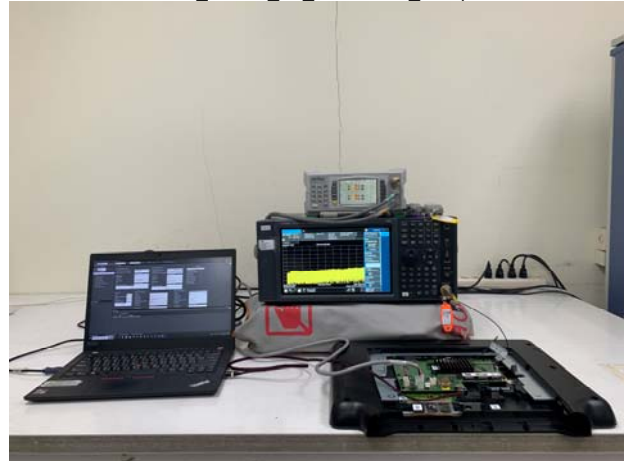
Part 15.247 LE Radiated Setup
