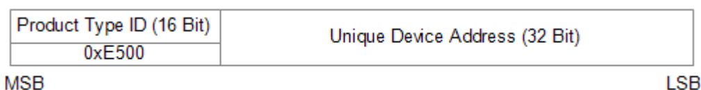
Figure 6 – BLE static source address structure
