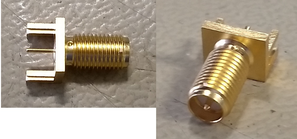
Figure 2: Reverse polarity SMA connector to be used for dipole antennas
