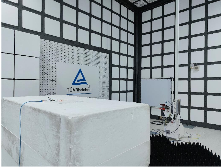
Photograph 14: Test Setup for Spurious Emissions (Back View 4)
