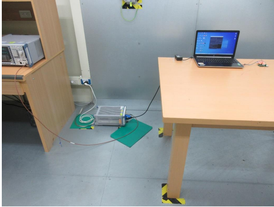
Photograph 32: Test Setup for Mains Conducted Emissions (Back View)
