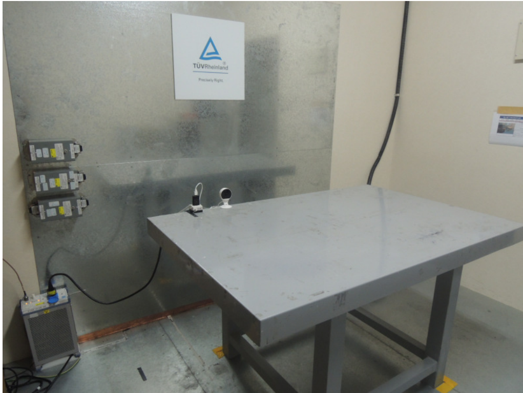
Photograph 7: Set-up for Mains Conducted testing (Front View)
