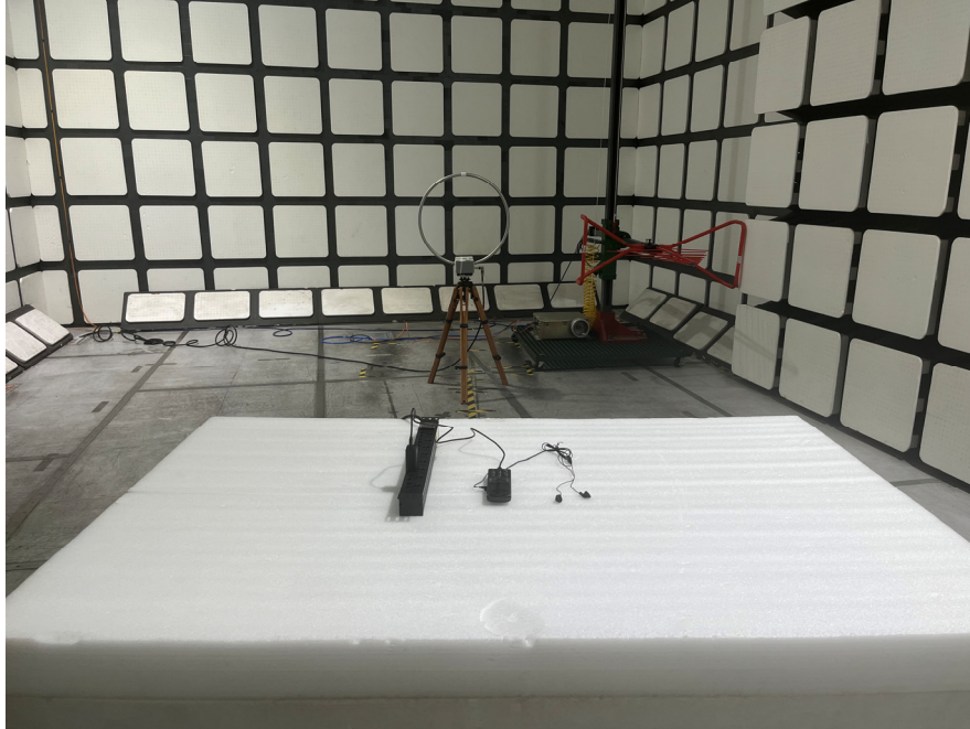
Radiated Emissions View (Below 30MHz)
