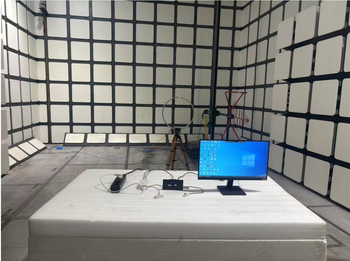
Radiated Emissions View (Below 30MHz) (For POE)
