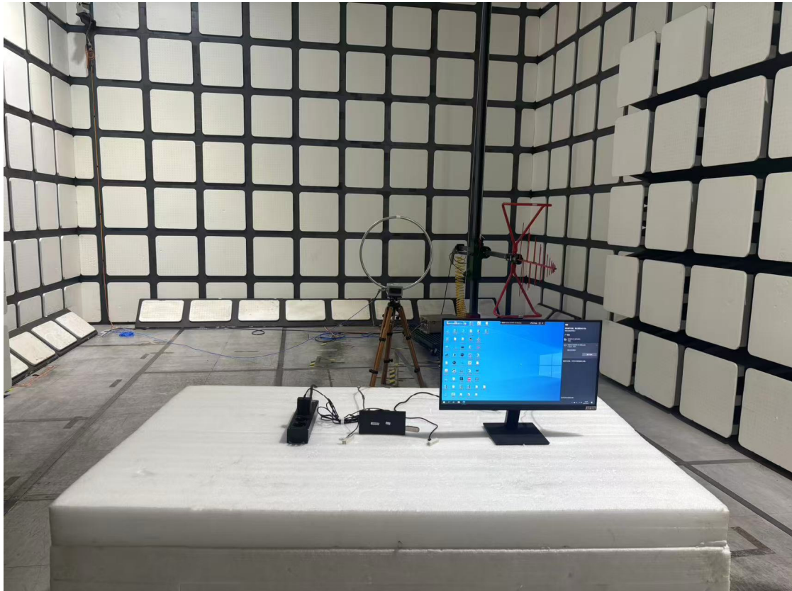
Radiated Emissions View (Below 30MHz) (For Adapter)
