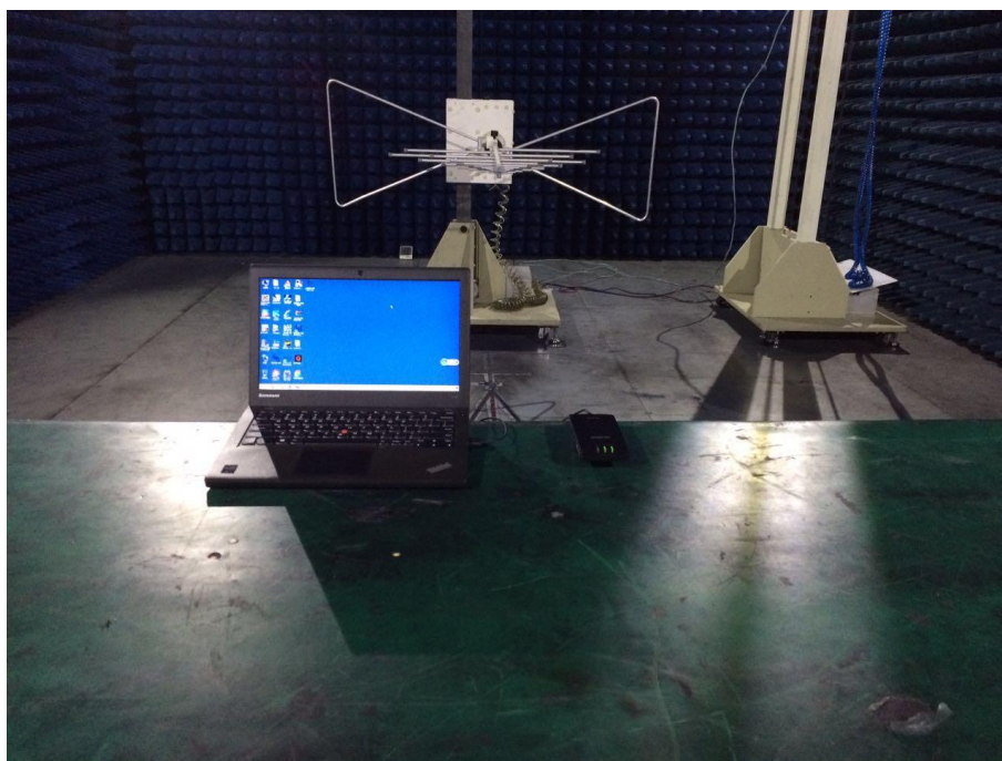
Radiated Emission test view (Frequency above 1GHz)
