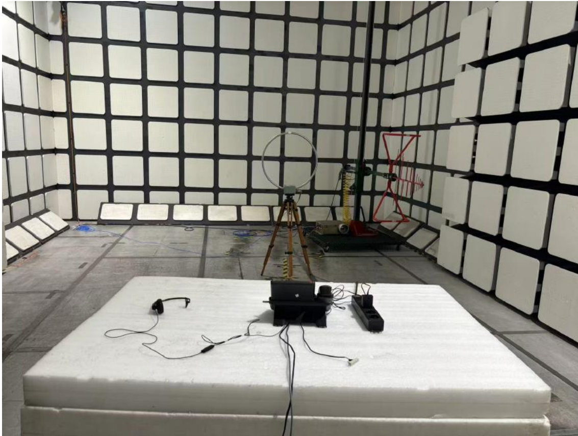
Radiated Emissions View (Below 1 GHz) (Adapter YLPS052000C1-US)
