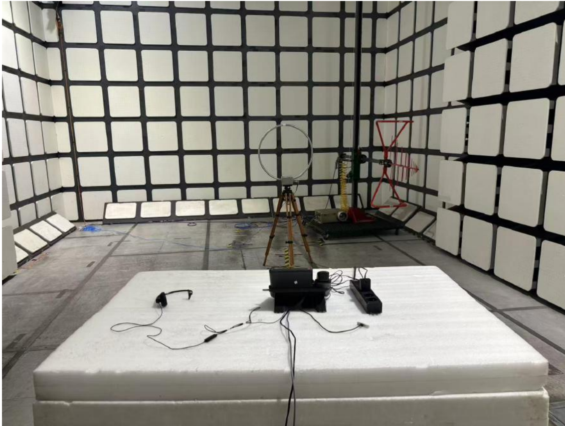
Radiated Emissions View (Below 1 GHz) (Adapter YLPS052000B1-US)
