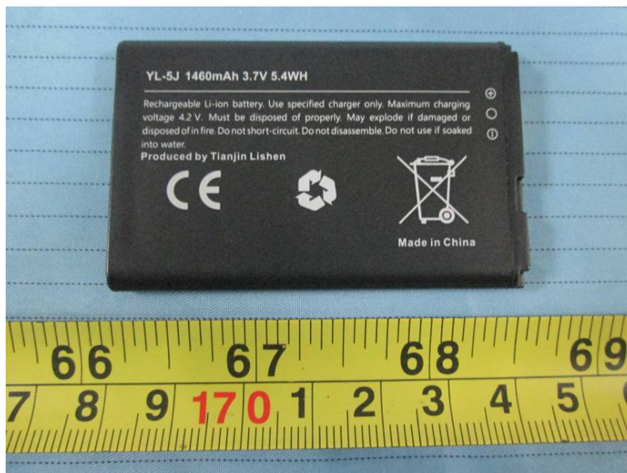
EUT – Battery Label View
