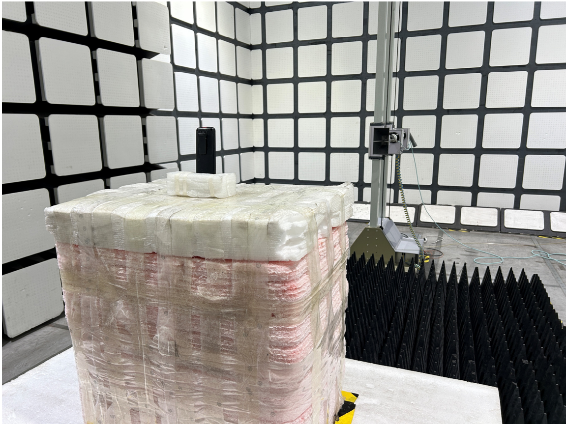
Radiated Emissions View (18-25 GHz)
