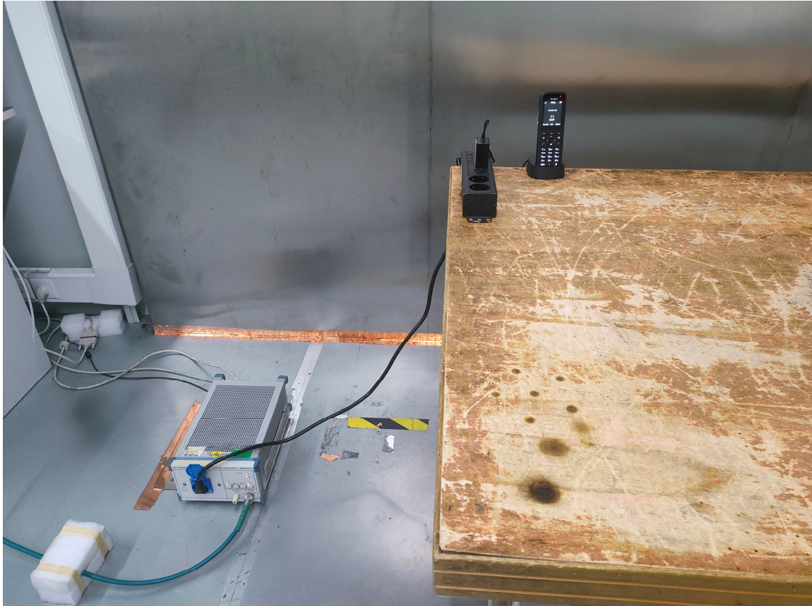
Conducted Emissions - Side View
