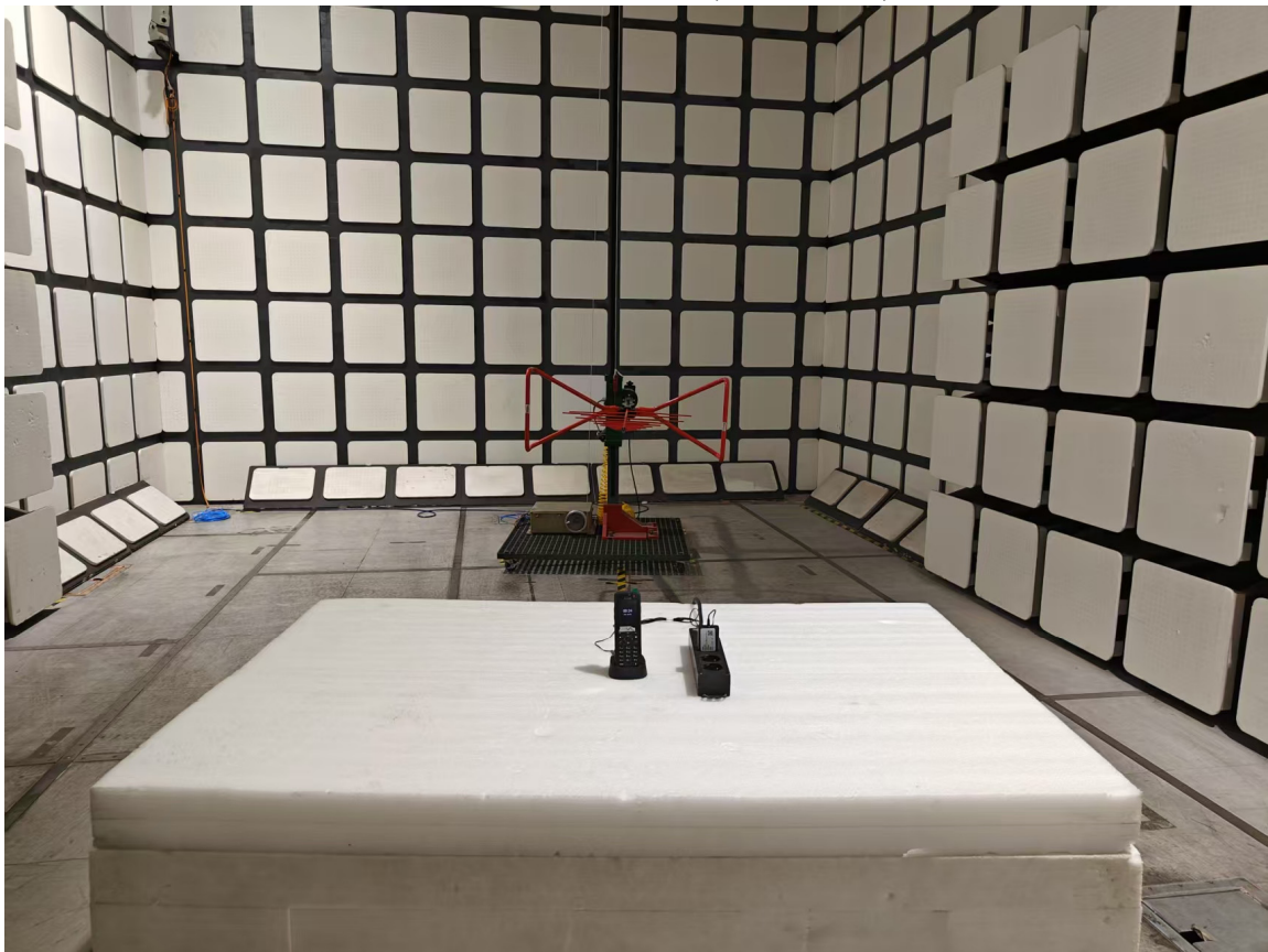
Radiated Emissions View (Below 1 GHz)
