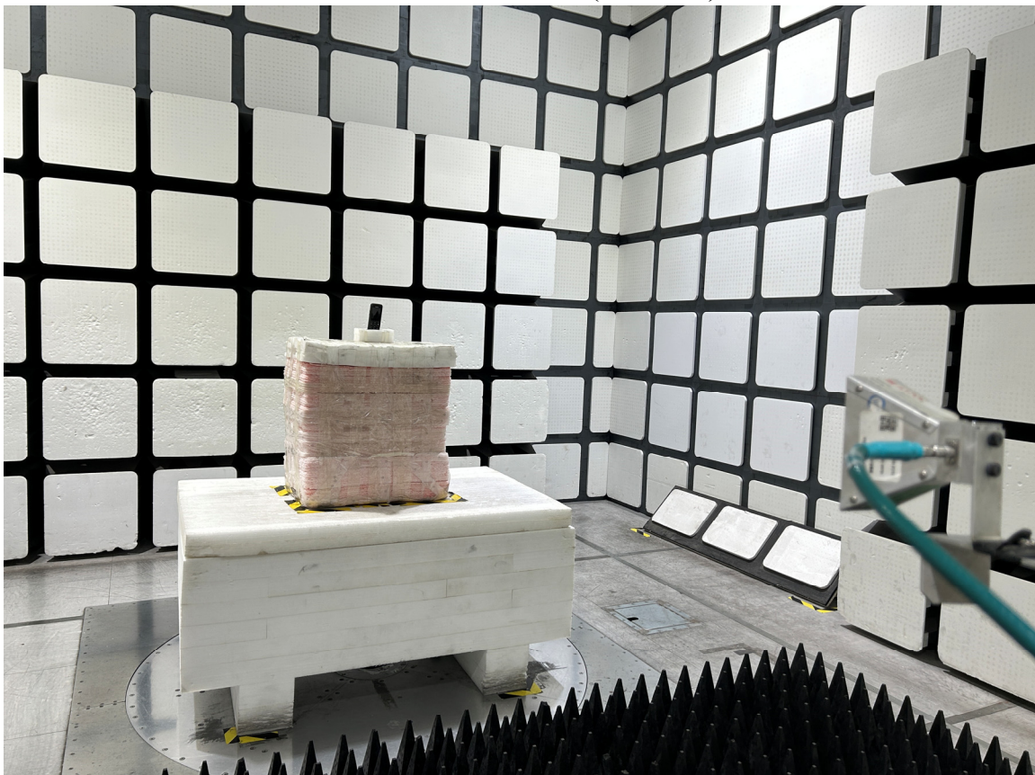
Radiated Emissions View (18-25 GHz)
