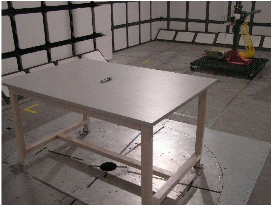
Radiated Emission - Rear View (Above 1GHz)
