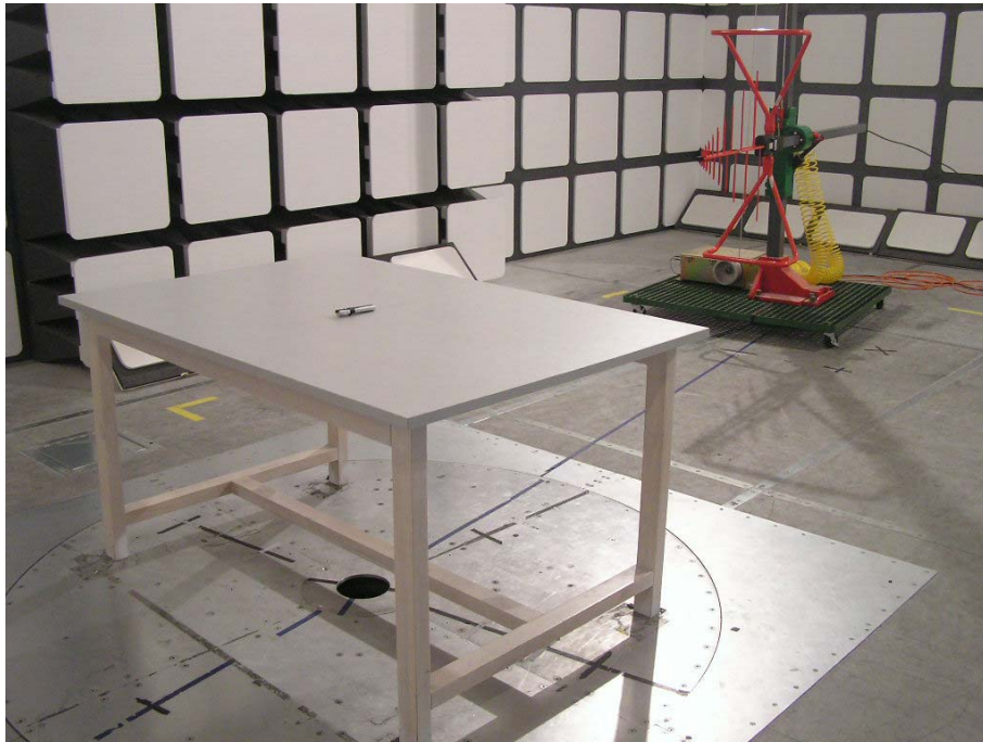
Radiated Emission - Front View (30-1000MHz)
