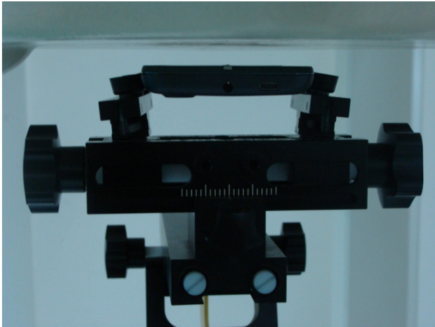
Front Side of the DUT with Phantom 1 cm Gap
