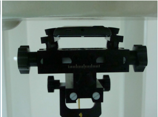
Back Side of the DUT with Phantom 1 cm Gap
