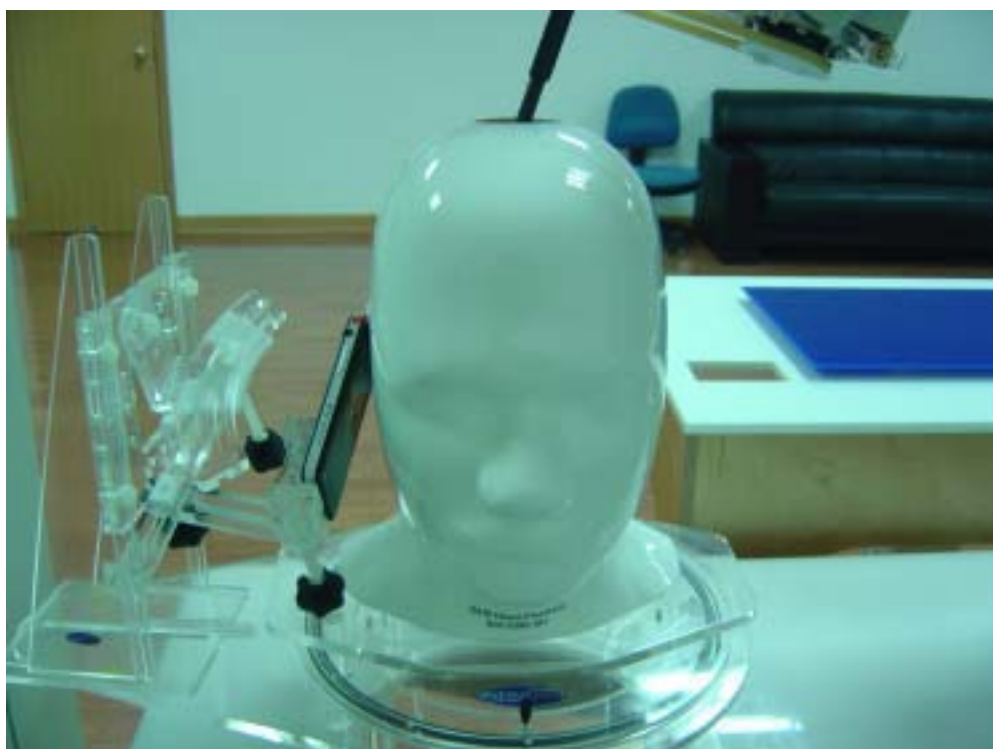
Fig.6 EUT Right Head Tilt15 Position
