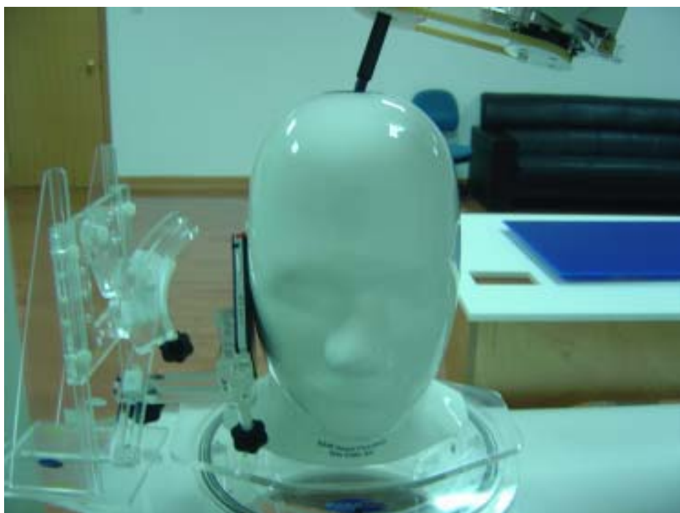
Fig.5 EUT Right Head Touch Cheek Position
