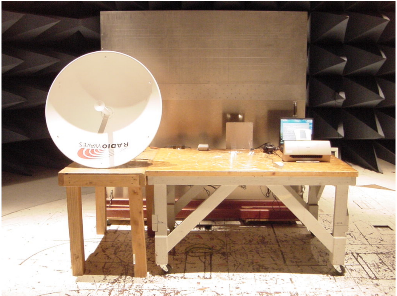
Photograph 2. Conducted Emissions Test Setup
