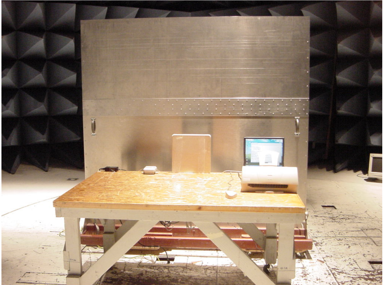
Photograph 2. Conducted Emissions Test Setup
