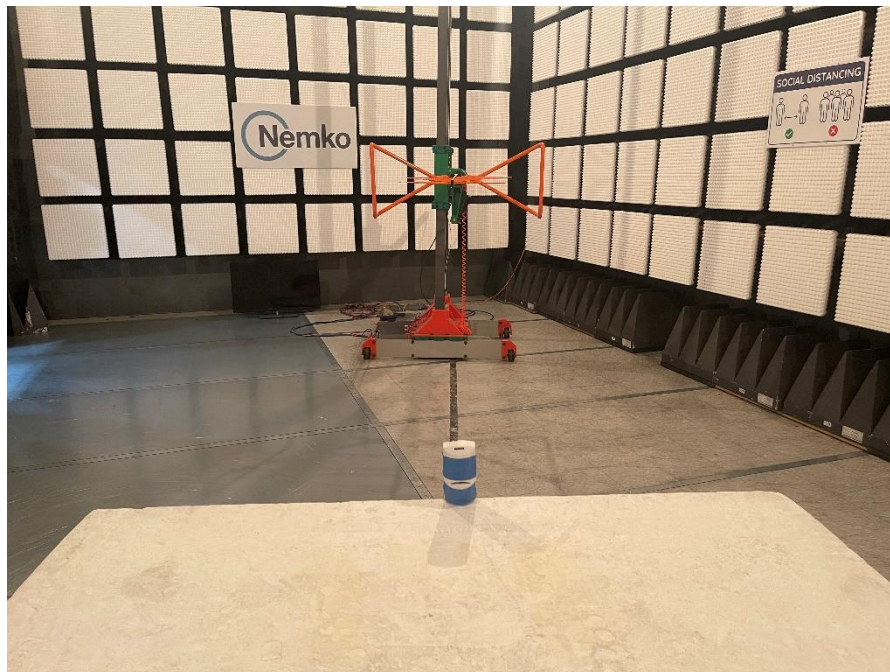
Figure 8.1-3: Radiated emissions setup photo – below 1 GHz
