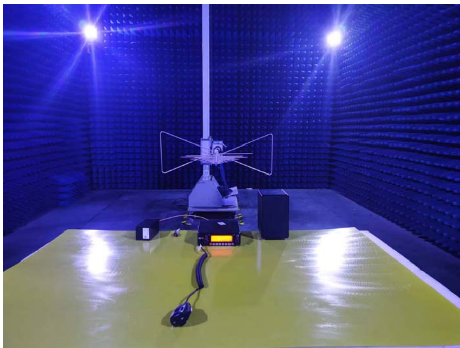
Photo of Radiated Emission Measurement (Below 1G)
