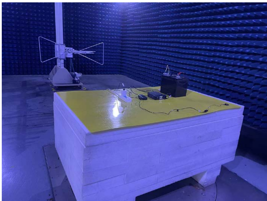
Photo of Radiated Emission Measurement Below 1GHz
