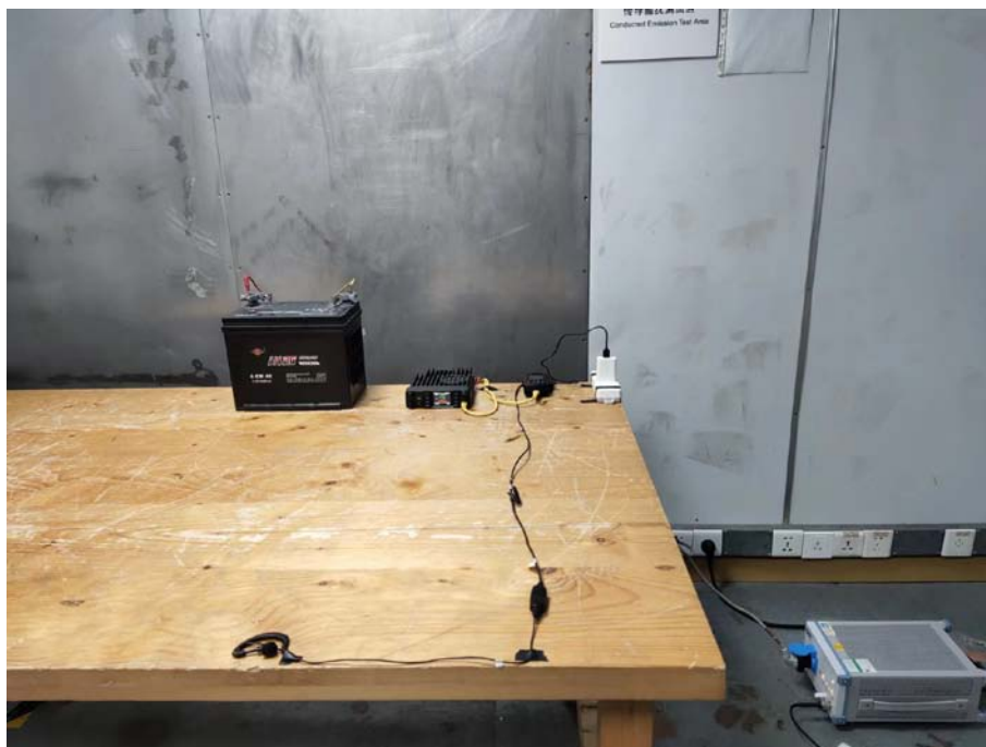
Photo of Conducted Emission Measurement
