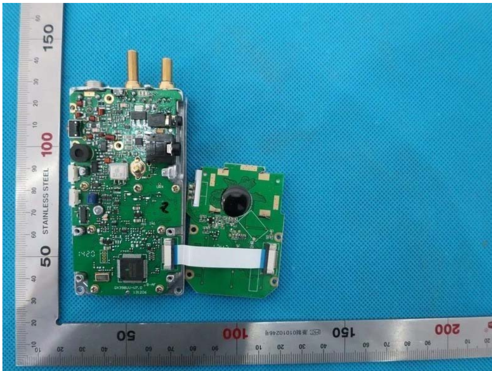
INTERNAL VIEW-1 OF EUT
