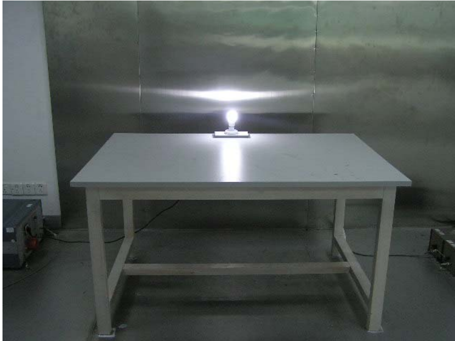
S-14W: Conducted Emission - Front View
