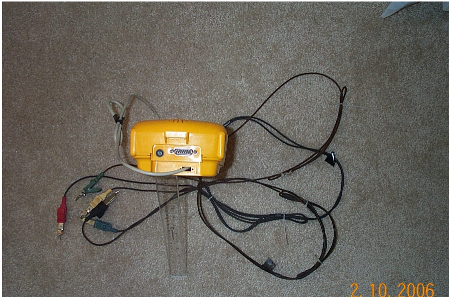
Figure 5, Top End View (DC power input connector is round dark object.)
