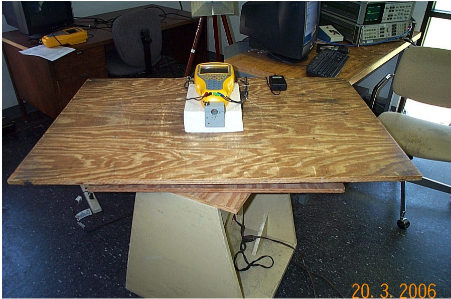
Figure 2, Spurious/Harmonics/Power/Bandwidth... > 1 GHz, Front The balun clamp visible at the front is used to hold the EUT upright.
