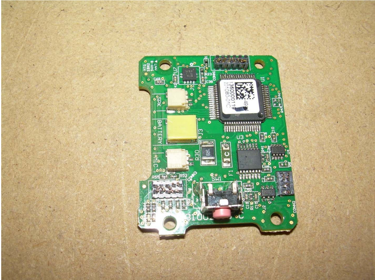
Photograph 12 – Top View of the Audio PCB
