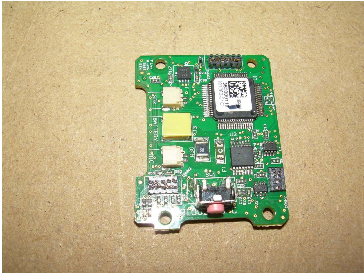
Photograph 12 – Top View of the Audio PCB
