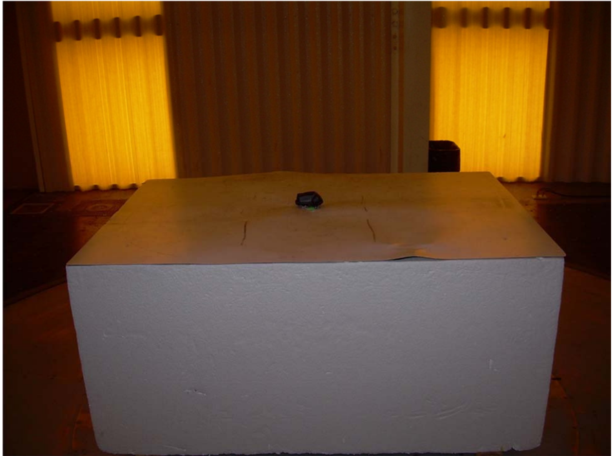
Front View Radiated Emission Test Set Up – Flat Configuration
