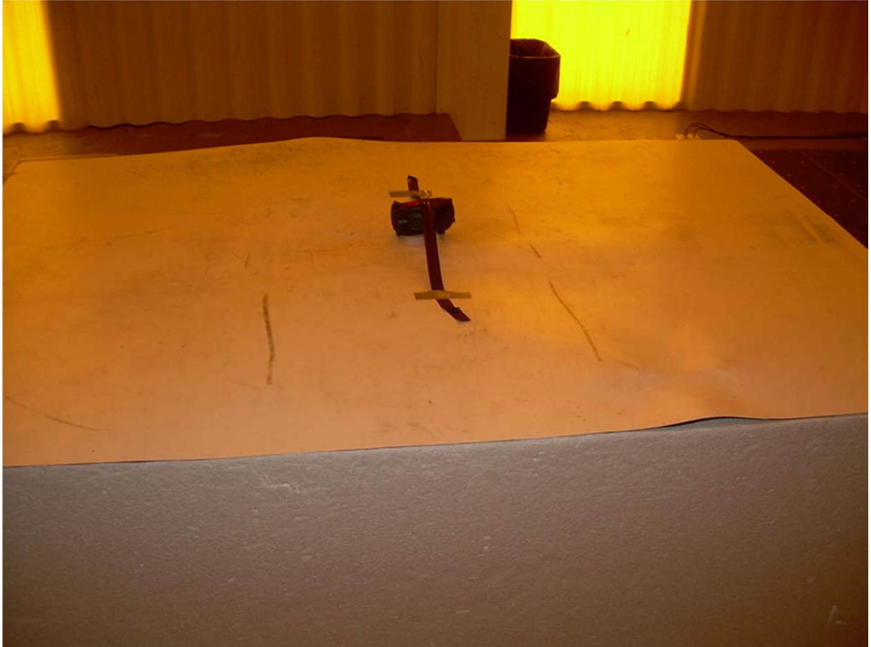
Front View Radiated Emission Test Set Up – On Edge Configuration
