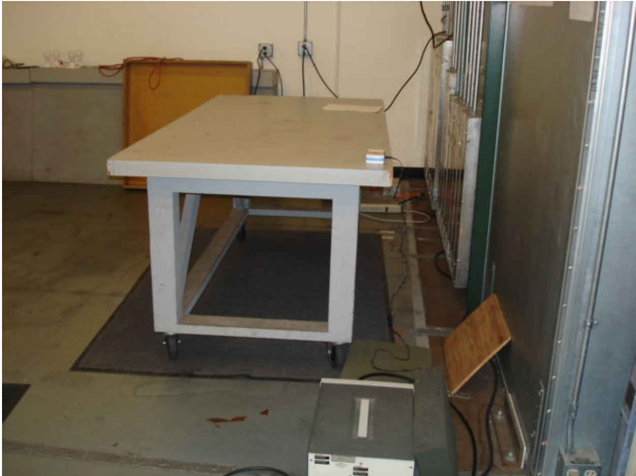
Remote, Conducted emission 2(15.107 / 15.207)
