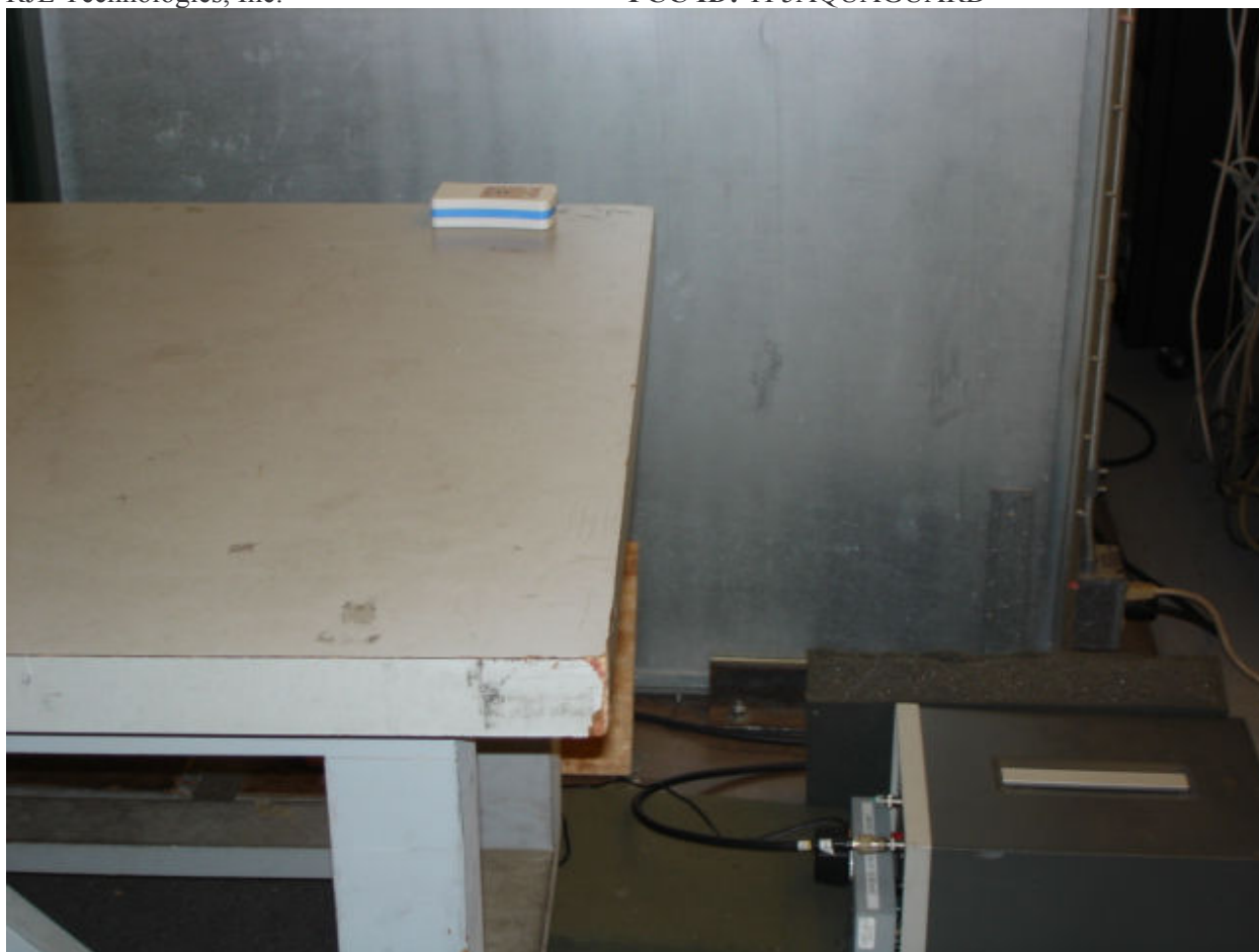
Remote, Conducted emission 1(15.107 / 15.207)
