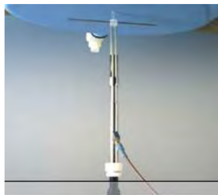
Photograph of the dipole Antenna
