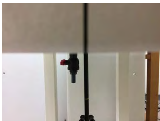
Fig.7 EUT Top side to flat phantom
