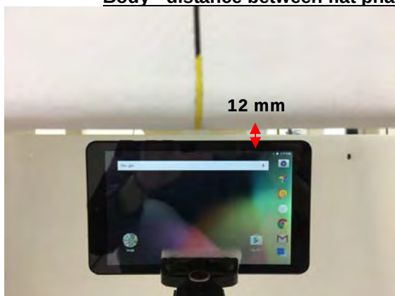
Fig.6 EUT Right side (12mm) to flat phantom
