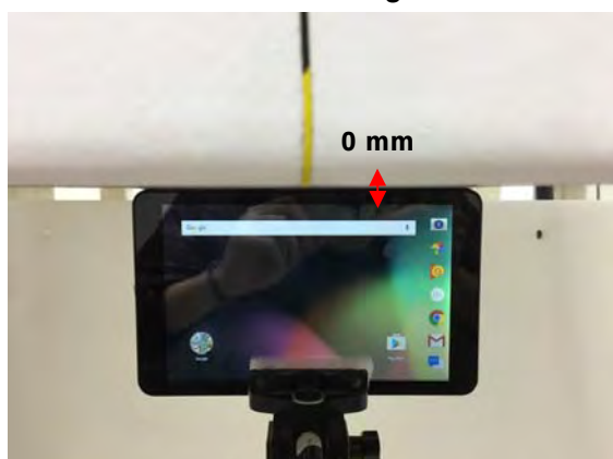
Fig.5 EUT Right side to flat phantom
