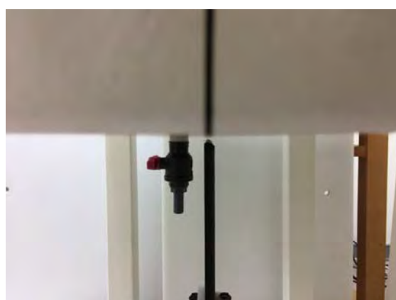
Fig.8 EUT Top side (5mm) to flat phantom
