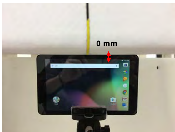
Fig.10 EUT Left side to flat phantom
