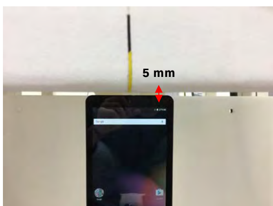
Fig.8 EUT Top side (5mm) to flat phantom
