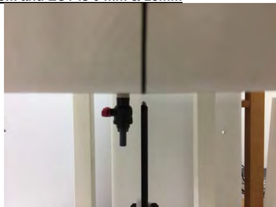
Fig.9 EUT Top side (15mm) to flat phantom
