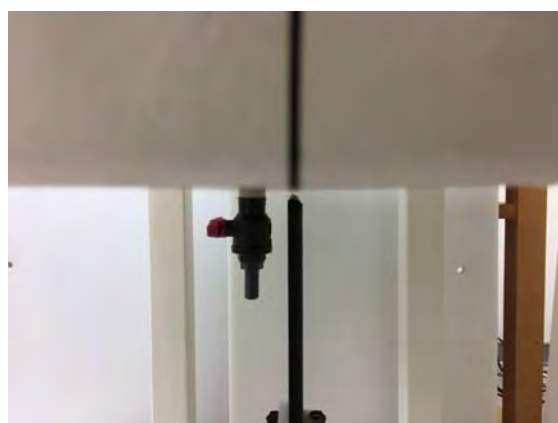
Fig.8 EUT Top side (5mm) to flat phantom
