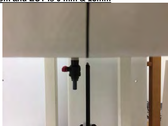
Fig.9 EUT Top side (15mm) to flat phantom
