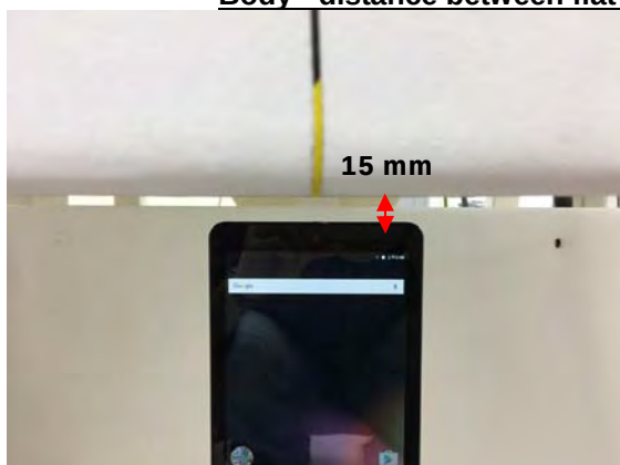
Fig.9 EUT Top side (15mm) to flat phantom
