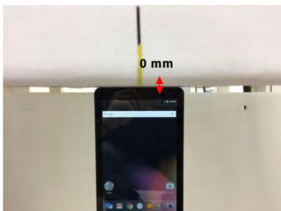
Fig.7 EUT Top side to flat phantom
