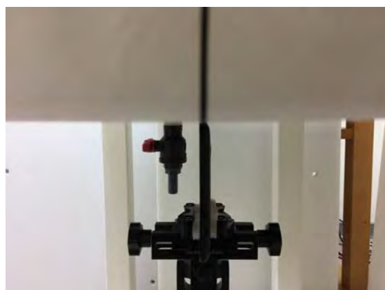
Fig.10 EUT Left side to flat phantom
