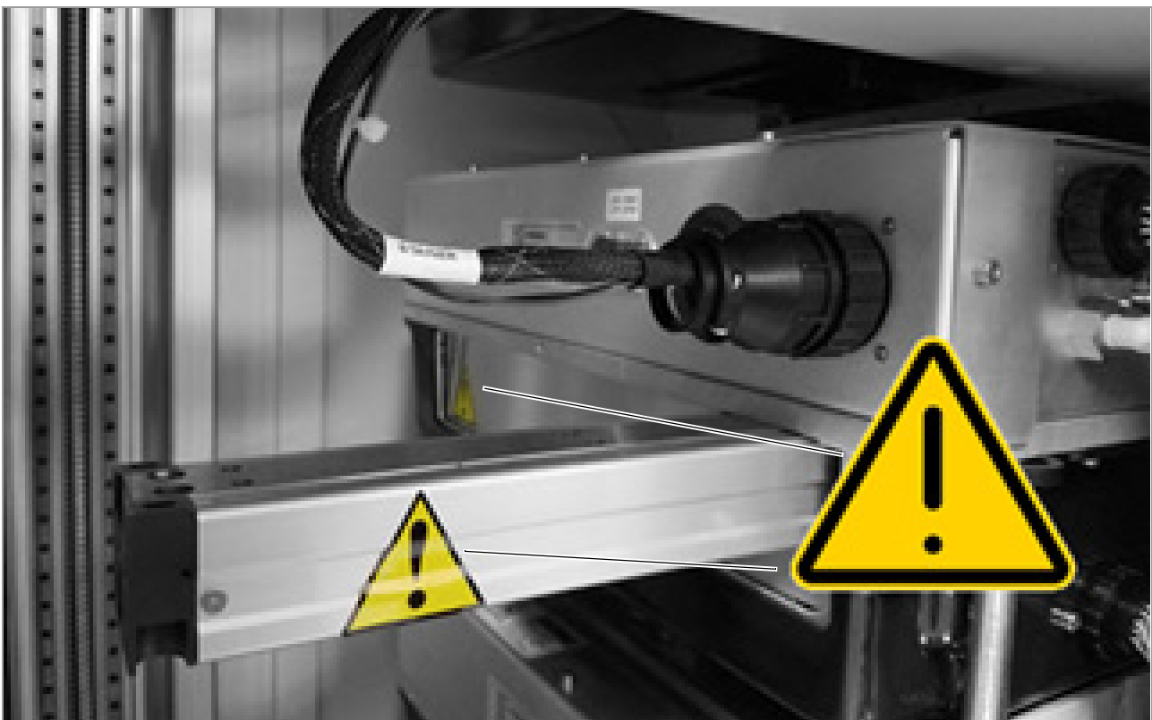
☐ Safety labels on each arm of the stainer crank and door in the transportation system module
